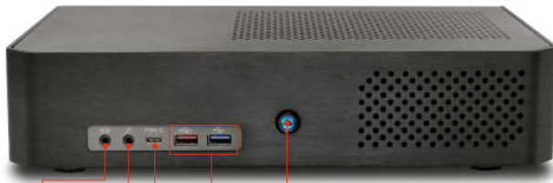
Line-Out Mic-In Type-C USB3.2 Power Button
