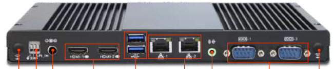
Antenna Hole DC-in HDMI 2.0 x 2 USB 3.0 x 2 LAN x 2 Line-out COM port x 2 Antenna Hole
